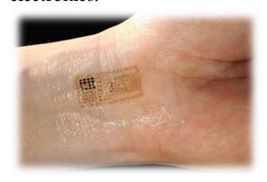
Flexible electronics also called flex electronics is a technology used for mounting electronic devices on a flexible plastic substrate such as polyimide and conductive polyester film.
