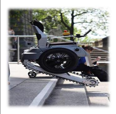
Argonault power wheelchair is a versatile mode of mobility with multi-functional ability. The wheelchair can lift up, down and can ascend/descend the stairs without any jerk.
