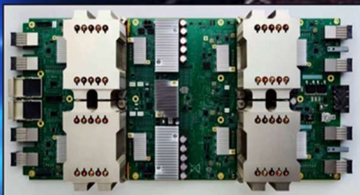
Figure 10: TPU2 with four TPU chips.
