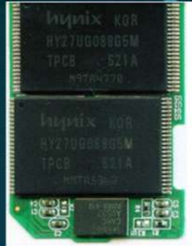
Inside a 2 GB SD card: two NAND flash chips (top and middle), SD controller chip (bottom)
